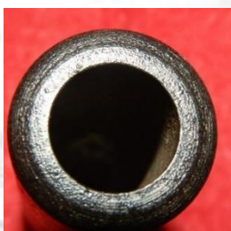
Open end of the metal tube for inserting the paper cartridges
