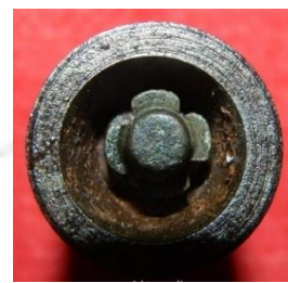
Percussion cap installed on nipple
