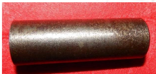
2¾ inch-long reusable metal tube used to hold paper cartridges. They were expensive to produce, heavy, and easily lost in the field
