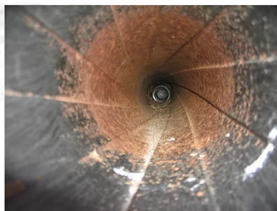
Rifling inside the barrel of a Parrott Gun
